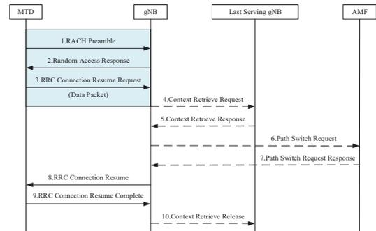
Fig. 3. Signaling diagram for the state transition from RRC INACTIVE to RRC CONNECTED.
