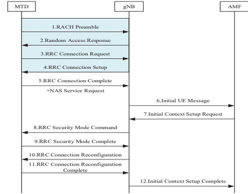
Fig. 2. Signaling diagram for the state transition from RRC IDLE to RRC CONNECTED.
