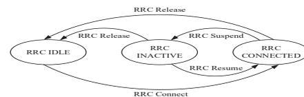
Fig. 1. RRC State Machine in 5G.
