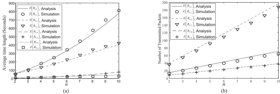
Fig. 4. (a) The expected buffering time for all SPs or PPs in one leasing or buffering period versus  $n$ . (b) The expected number of SPs or PPs transmitted in one leasing or buffering period versus  $n$ .
