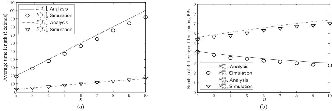
Fig. 3. (a) The expected time length of one leasing or buffering period, i.e.,  $E[T_L]$  or  $E[T_B]$ , versus  $n$ . (b) The expected number of buffering and transmitting PPs at the beginning of one leasing or buffering period, i.e.,  $N_{P,L}^{(0)}$  or  $N_{P,B}^{(0)}$ , versus  $n$ .
