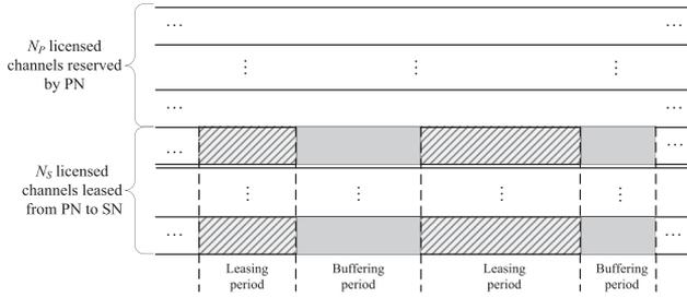
Fig. 1. In the proposed traffic-adaptive spectrum leasing (TASL) scheme, the infinite time of the  $N_S$  licensed channels leased from the PN to the SN are synchronously divided into leasing and buffering periods with variable time lengths, which can fully adapt to the real-time secondary traffic.
