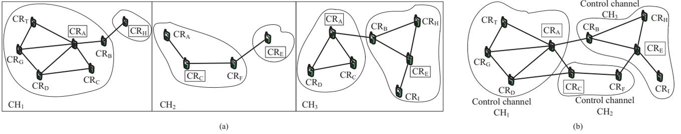
Fig. 3. The layered clustering results of the CRAHN in Figure 1 at each of the 3 spectrum channels  $CH_1$ ,  $CH_2$  and  $CH_3$  are depicted in (a) and merged into a final clustering result in (b) via first eliminating redundant clusters and then merging effective clusters, where each cluster is surrounded by a circle and each node in a square denotes a cluster head.
