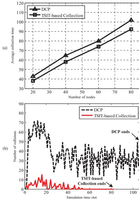
Fig. 5. (a)The average time for distributed collection of network information; (b)the number of collisions in distributed collision.
