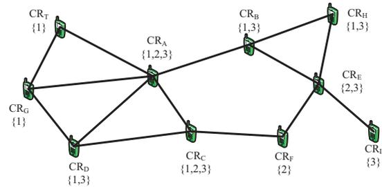
Fig. 1. A cognitive radio ad hoc network with heterogeneous spectrum, where the number below each node represents the label of an available channel .
