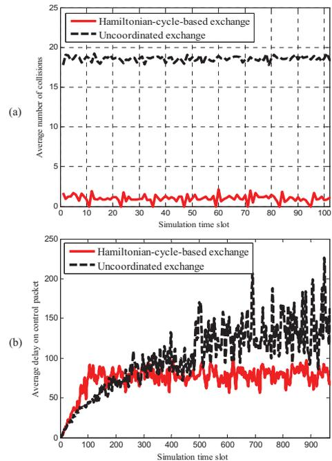
Fig. 7. Comparison between Hamiltonian-cycle-based and uncoordinated control information exchanges among clusters. (a)Average number of packet collisions; (b)Average delay of control packets
